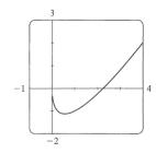
(b) Since F(0)=1, we can start our graph at (0,1). f has a minimum at about x=0.5, so its derivative is zero there. f is decreasing on (0,0.5), so its derivative is negative and hence, F is CD on (0,0.5) and has an IP at  $x\approx 0.5$ . On (0.5,2.2), f is negative and increasing (f') is positive, so F is decreasing and CU. On  $(2.2,\infty)$ , f is positive and increasing, so F is increasing and CU.
